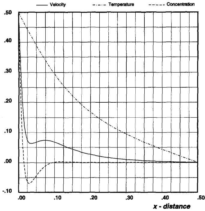
Fig. 12. Vertical velocity, temperature and concentration profiles in the horizontal midplane ( Ra^* = 100 ; Da = 10^{-7} ; A = 1 ; N = 2 ; Le = 100 ).
